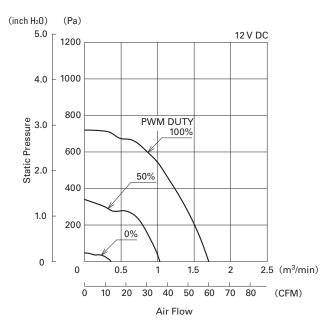
Fig. 6: Air flow vs static pressure characteristics at individual PWM duty cycle(9CRA0612P0S001)
