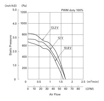
Fig. 4: Air flow vs static pressure characteristics (9CRA0612P0S001)
