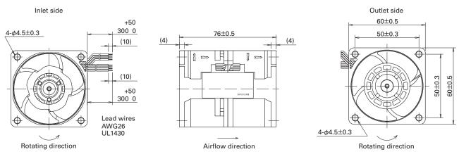
Fig. 2: "San Ace 60" CRA type dimensions (unit: mm)
