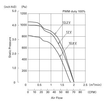
Fig. 3: Air flow vs static pressure characteristics (9CRA0612P0G001)
